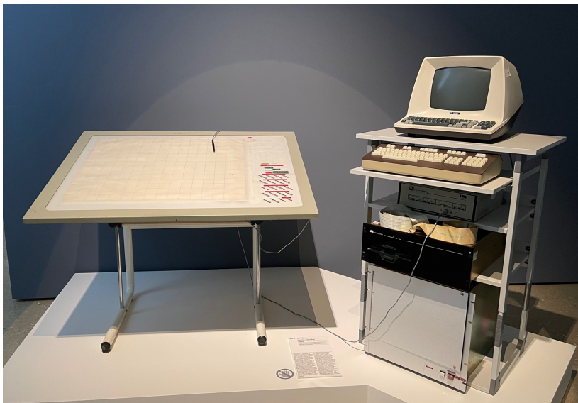
A 1986 UPIC digital computer system for sound creation by Iannis Xenakis
